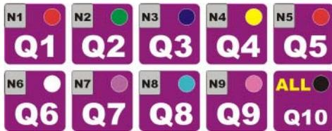
**Fixture Select buttons** are multi function buttons. They will be used to select a fixture, Change networks and select a color preset.
