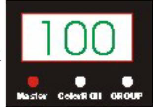
**Master** indicator will light when master value is below 100%. This will alert the user that the master is not at full intensity.
